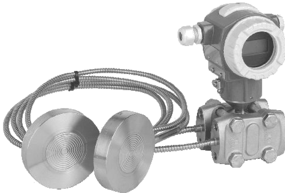
Figure 1-2: dP Transmitter with Filled System Connecting to Remote Diaphragms (Courtesy: Endress + Hauser)
