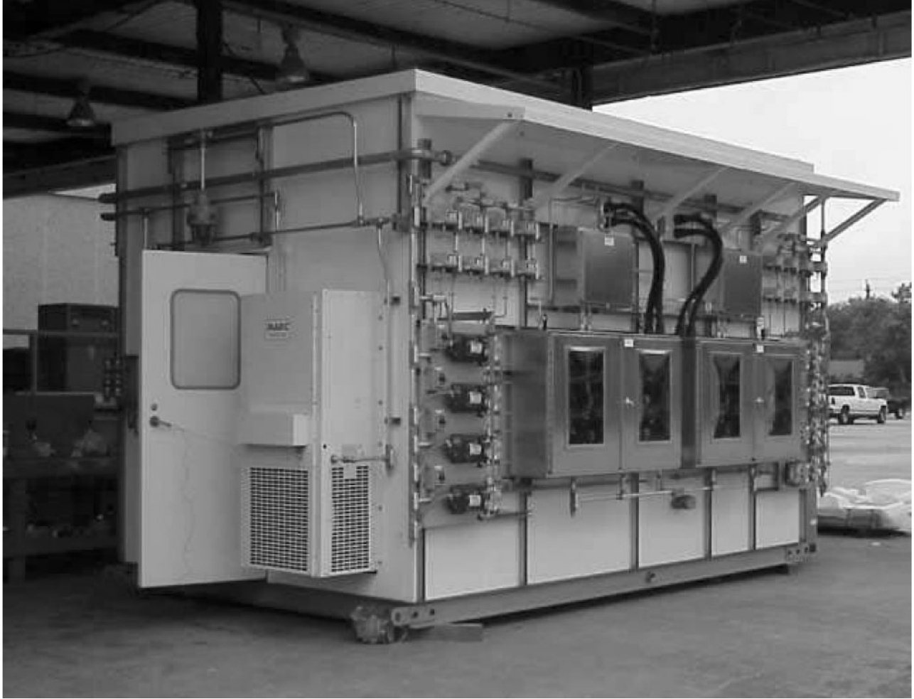
Figure 2-4: An Outside View of an Analyzer Shelter (Courtesy of Technical Automation Service Corp. (TASC))
